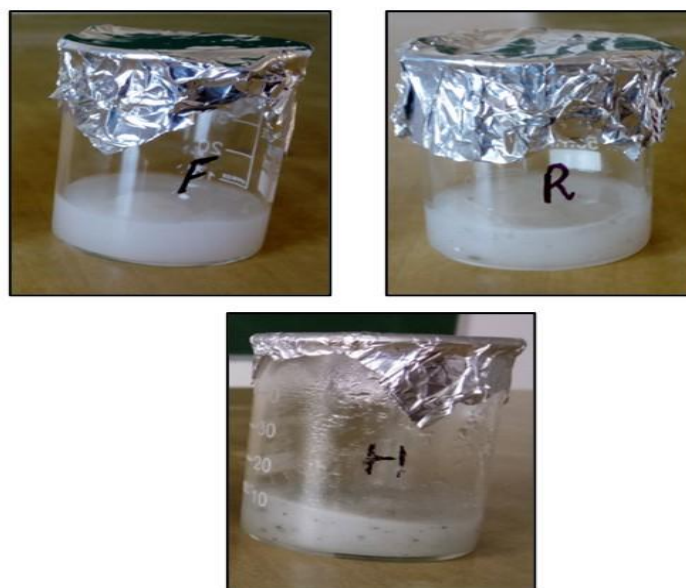
Figure 15 Changes in physical appearance after 3 months. F, Freeze conditions; R, Room Conditions; H, High Temperature conditions.
